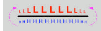
Rear view of a wing showing formation of wingtip vortices as air flows from high pressure below to low pressure above.
